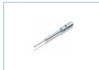
Disc stylus 1 mm Order no.: 101-030-010 single-item, \varnothing 1 mm / R: 25 \mu m / A: 2 x 12°, including extension (made of one piece - carbide), length 25 mm from front edge of quick-release fastener
