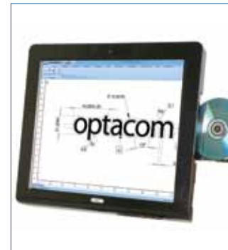
Panel PC 19" with touchscreen IP64 40 GB SSD and Windows XP Professional Intel Celeron Mobile 1.0 GHz, 1 GB DDR 2 Resolution 1280 x 1024 pixels Order no.: 101-217-310
