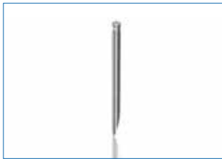
Stylus tip 59.5 mm Order no.: 101-010-001 made of carbide, Ø 3.5 mm / R: 25 µm / A: 12° Mahr compatible (6851517)
