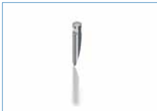
Stylus tip 20.5 mm Order no.: 101-010-003 made of carbide, Ø 3.5 mm / R: 25 µm / A: 12° Mahr compatible (6850289)
