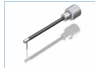
Miniature stylus arms for removable stylus tip Ø 1 mm Order no.: 101-010-060 including quick-release fastener, standard length 50 mm (other lengths upon request); delivery without stylus tips!
