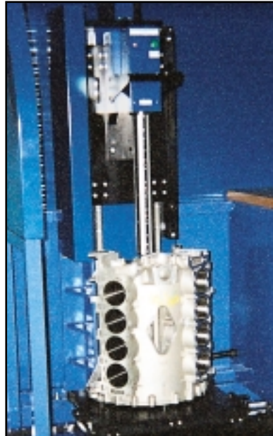
Talyseries Roundness system configured for the measurement of crank bores. This system has ten gauges otherwise all other facilities are as denoted below.
