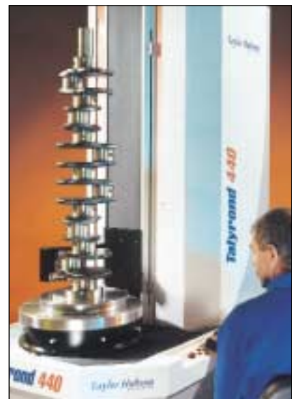
the massive worktable is powered by dual, high torque, direct drive motors for accurate positioning of centric loads to 225Kg (495lbs)
