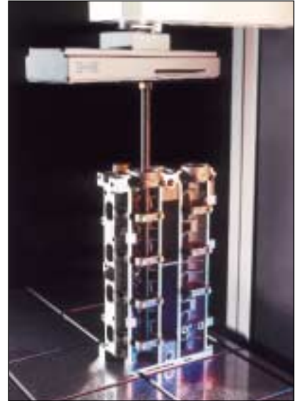
engine blocks can be mounted vertically for the measurement of crankshaft and camshaft bores using a suitable gauge extension arm
