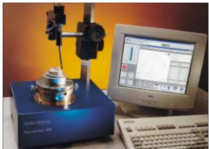
computer assisted center and leveling powered by ultra software
