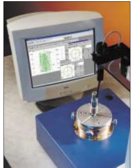
cylindricity analysis with Talyrond 131
