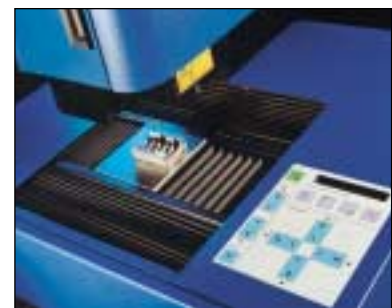
Talyscan 150 (detail of X - Y traverse stage)
