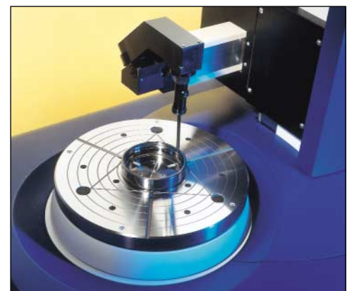
Talyrond roundness measuring instrument
