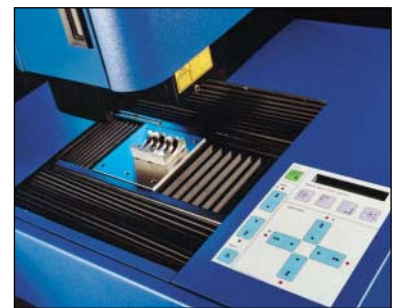
Talysurf CLI (detail of X - Y traverse stage)
