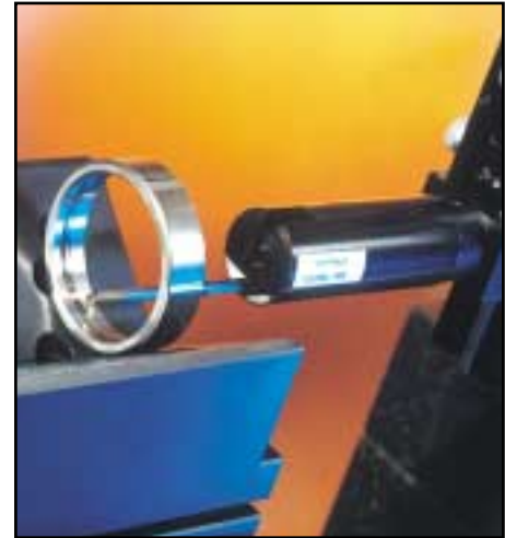
skidless tracing arms provide access to internal features such as ball tracks and ring grooves
